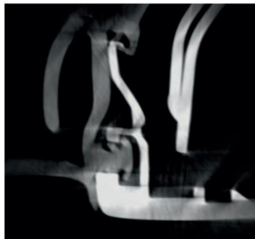
Figure 10 – CT slice orthogonally through the doorframe (on the right), clearly visualizing the door's rubber seal (on the left) and how it snaps into the metal structures.
