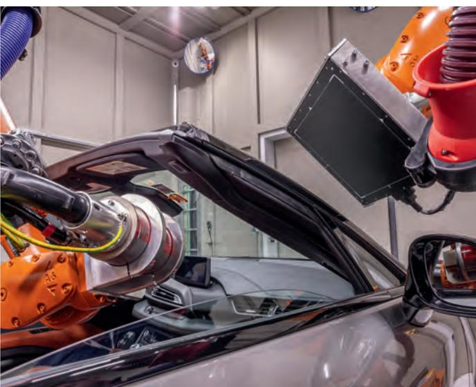
Figure 2 – Robots positioning X-ray source and detector at the A-pillar of a BMW i8 Roadster.
