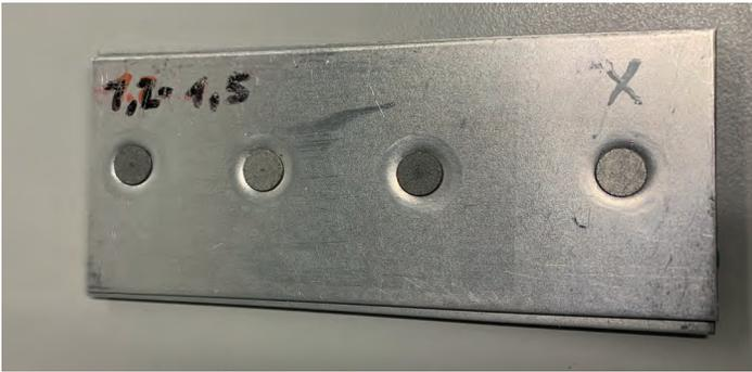
Figure 3 – specimen: rivet joint plates, 110 mm x 50 mm.
