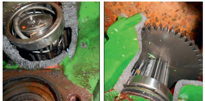
Figure 1. Characteristic consequential damage of a gearbox after gear damage or bearing damage
