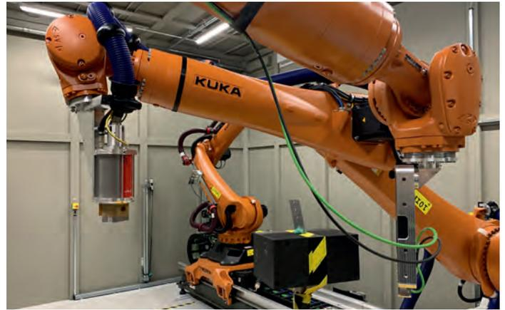
Figure 4 – unobstructed specimen in RoboCT setup with robots at maximum angle of 120°.
